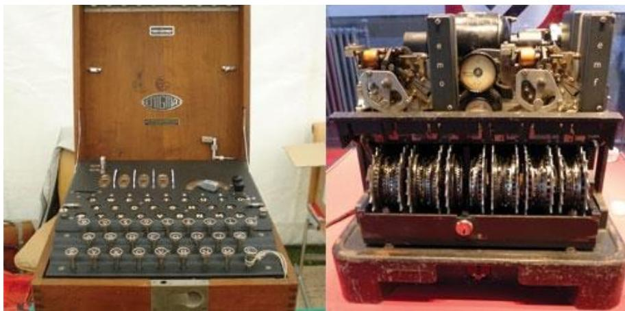
*Enigma and Lorenz-The four-rotor naval Enigma (left) used Morse code and the 26-letter alphabet, whereas the vastly more complex German Lorenz cipher encrypted messages that were sent by radio teleprinter using Baudot code. Tutte is credited with cracking the Lorenz code.*
