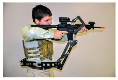
The Army Research Laboratory is developing a "third arm" passive mechanical appendage that could lessen Soldier burden and increase lethality. Weighing less than 4 pounds, the device attaches to a Soldier's protective vest and holds their weapon, putting less weight on their arms and freeing up their hands to do other tasks. (Photo Credit: Courtesy photo)
