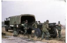
to Shilo, the Regt usually flew in and drew equipment from Shilo's resources. Note the ramp on the side of the tractor. This tractor is from Shilo and was normally used for the L5 light gun. The ramps were used to portée the L5. They were winched up the ramps into the back of the truck.
