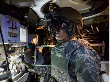
IronVision displays 360 degree, high-res imagery from data collected from digital sources in and around the vehicle. Photo: Elbit
