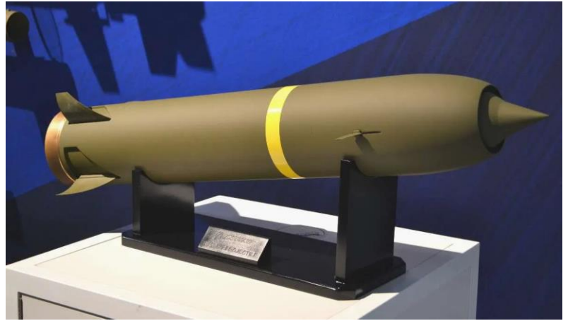
Mock-up of the Boeing-Nammo ramjet artillery round design. Joseph Trevithick
