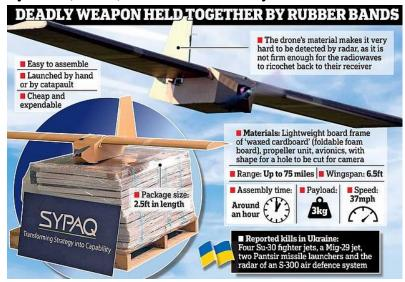
The drones, believed to be virtually undetectable by radar, can fly for 75 miles at 37mph and are capable of carrying up to 3kg of load
