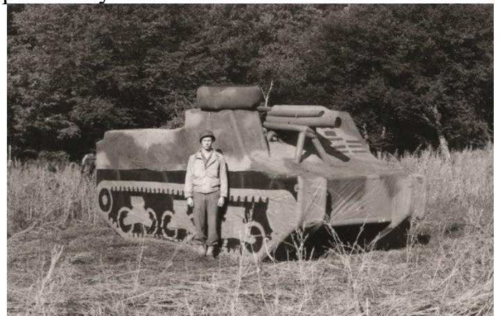
An inflatable M7 Priest set up in a field on maneuvers in 1944.
