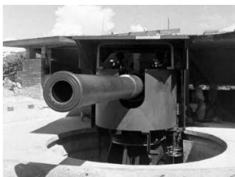
The Labrador Battery No1 Gun with a locally made shield & overhead cover.
