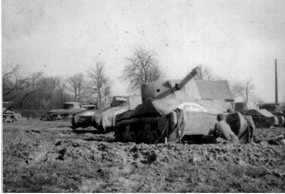
Just a few of the 603rd Camouflage Engineer Battalion's many inflatable tanks.
