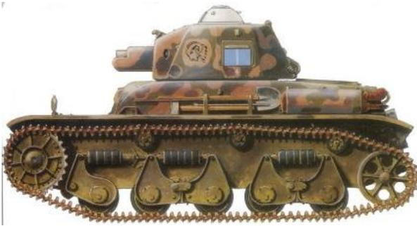
resemblance to its rival, the Hotchkiss H35. They shared the same APX turret, the three-module hull construction and placement for the driver and engine. However, their dimensions differed, as well as the placement of the hull casemate, placed further to the rear for the Renault and, most obviously, the drivetrain. The hull, as stated above, was made of three main prefabricated cast sections bolted together, while on
