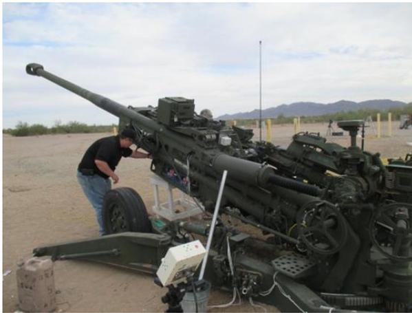
*Personnel checking and securing instrumentation on the Extended Range M777A2 in-between firing occasions.
