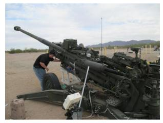
Personnel checking and securing instrumentation on the Extended Range M777A2 in-between firing occasions. Courtesy photo (Photo Credit: U.S. Army)
