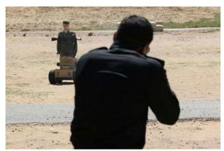
This moving, semi-autonomous robotic target is being tested by the Marine Corps for use on small arms ranges. (Marathon)
