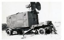
This is an Anti-Aircraft Artillery Radar unit used by the 43<sup>rd</sup> MAA in the mid-50s. We believe it is a No 4, Mk 7 unit.
