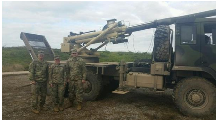
The Brutus is a 155mm artillery piece mounted on a 5-ton truck by AM General, using Mandus Group's "soft recoil" technology. It was recently fired at the Fires Center of Excellence Maneuver Fires Integration Experiment at Fort Sill, Oklahoma. (Army)
