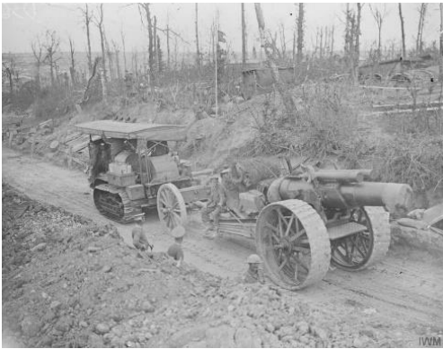
8" Howitzer towed by a Holts Tractor. These are the "Caterpillars" mentioned by Blackadder IWM Q 4322
