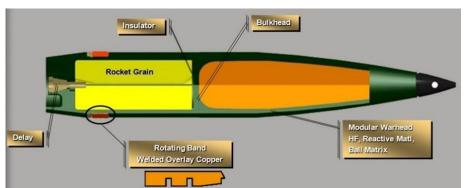
The XM1113 consists of a high fragmentation steel body with a streamlined ogive, the curved portion of a projectile between the fuze well and the bourrelet, and a high performance rocket motor. The projectile body is filled with insensitive munition high explosive and a supplementary charge. On gun launch, propellant gases initiate a
