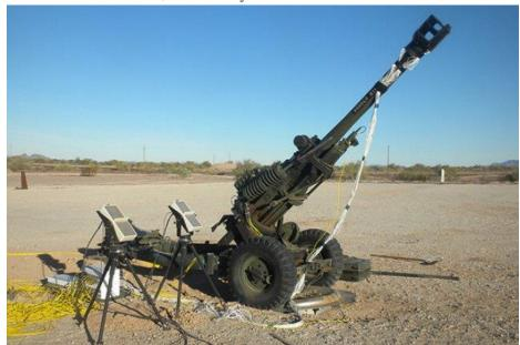
The M119 105mm howitzer, outfitted with the LBOP muzzle brake, ready for live-fire testing at the Yuma Proving Ground in Arizona. (Photo Credit: Courtesy
