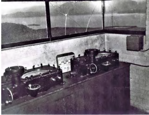
9H – Searchlight Controls. The direction and elevations of the searchlights were controlled from the BOP circa 1943 and later. 15FdMuseum997.001.082A
